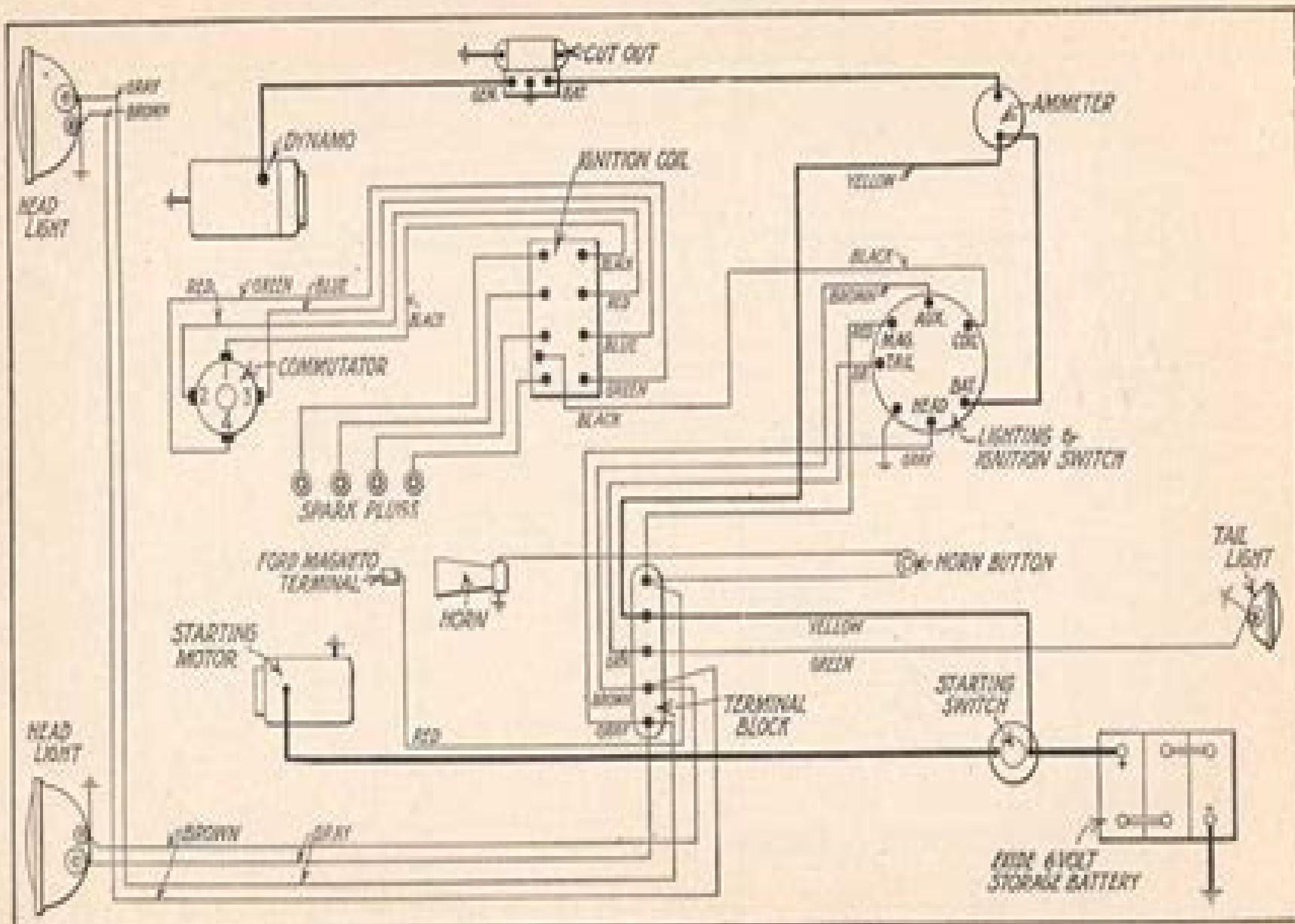
Fig. 87. Wiring Diagram with Cutout on Dash
